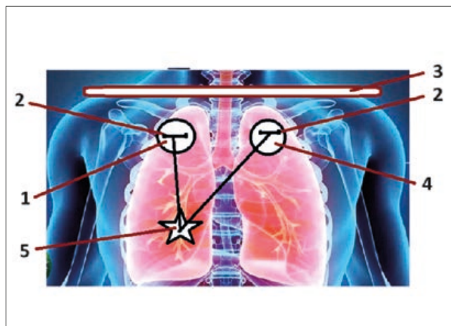
Fig. 1. Scheme of positioning of the pathological process when using the acoustic monitoring device «Trembita—Corona»: 1 — first listening point; 2 — pair of receivers; 3 — line connecting the patient's clavicles at two listening points; 4 — second listening point; 5 — pathological process
